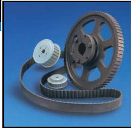
Martin timing pulleys are manufactured to fit the old standby trapezoidal profile and are stocked in minimum plain bore, taper bushed and QD bushing styles.
