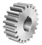
**Change Gears:** Standard steel change gears and bushings stocked in all tooth sizes for 20, 16, 12, 10, and 8 Diametral Pitch - 14 1/2° pressure angle.
