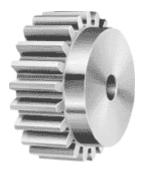
**Spur Gears:** Steel spur gears in 20 through 2 Diametral Pitch - 14 1/2° pressure angle stocked. Other circular, metric, or D. P. sizes made-to-order in 14 1/2°, 20° or other pressure angles from steel, nylon, phenolic, bronze, cast iron or other materials up to 96" diameter. Internal gears and ground external profiles may be provided subject to equipment limitations.
