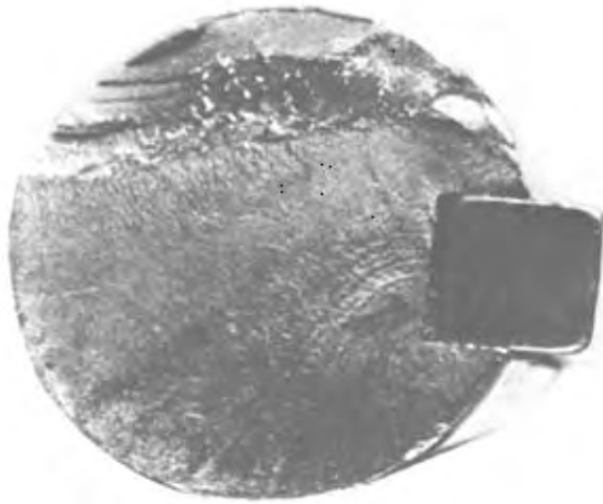
FIG. 3.4 (548-1) SHAFT FRACTURE (KEY AND KEYWAY ASSOCIATED)
