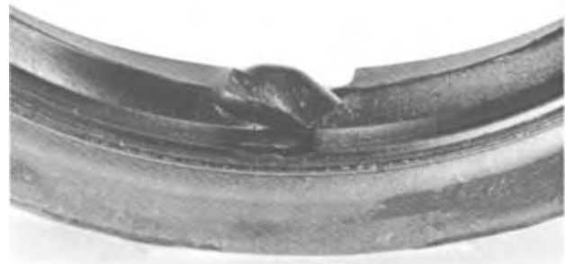
FIG. 5.2 (2342-37C) CUT AND TURNED UNDER LIP
