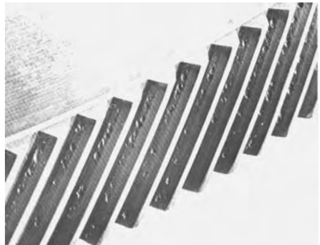
FIG. 2.15 (13-162) SPALLING (THRU HARDENED GEAR)
