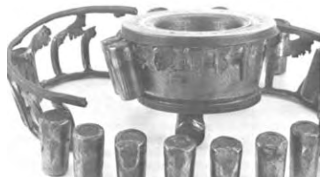
FIG. 4.3 (2342-30C) WELDING OF ROLLERS
