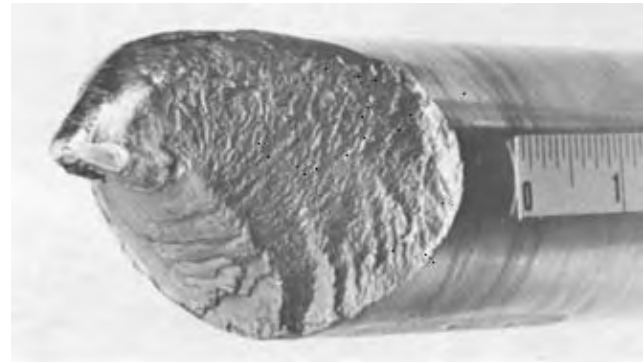
FIG. 3.2 (2342-26C) TORSIONAL FRACTURE
