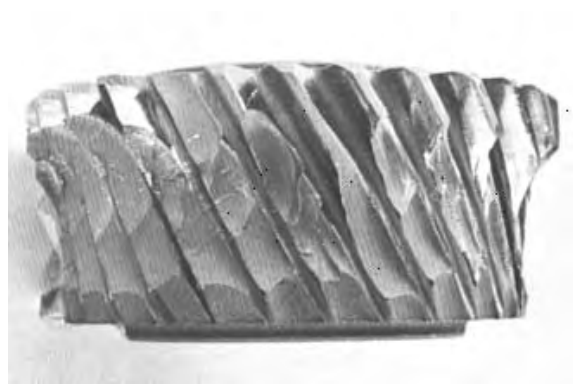
FIG. 2.46 (683-14) TOOTH FRACTURE FROM BEARING FAILURE
