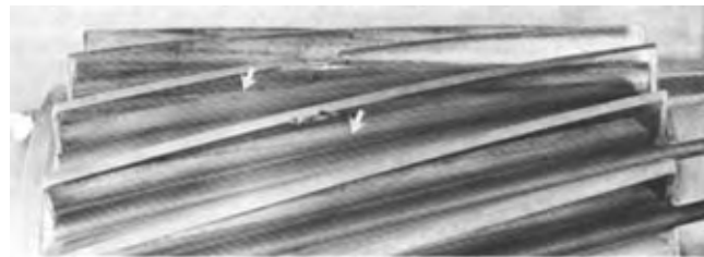
FIG. 2.32(2342-13C) WAVY TOOTH WEAR
