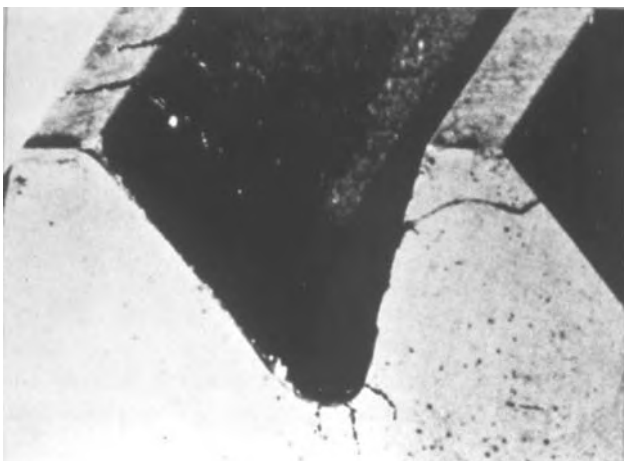
FIG. 2.47 (2342-22C) QUENCH CRACKS (THRU HARDENED MATERIAL)
