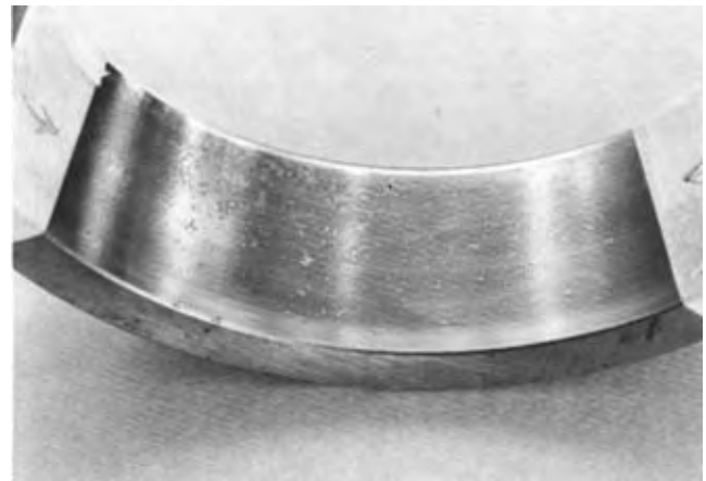
FIG. 4.2 (2342-29C) DEBRIS DENTING
