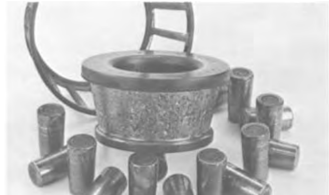
FIG. 4.8 (2342-35C) CAGE WEAR AND ROLLER END WEAR
