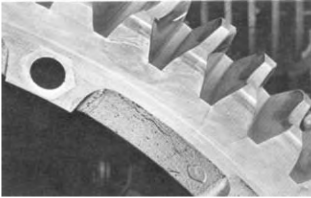
FIG. 2.45 (2342-21C) WORM WHEEL TOOTH FRACTURE
