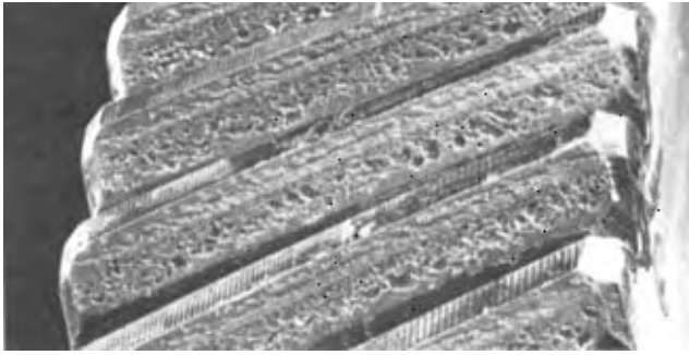
FIG. 2.16 (2342-7C) SPALLING (THRU HARDENED GEAR)
