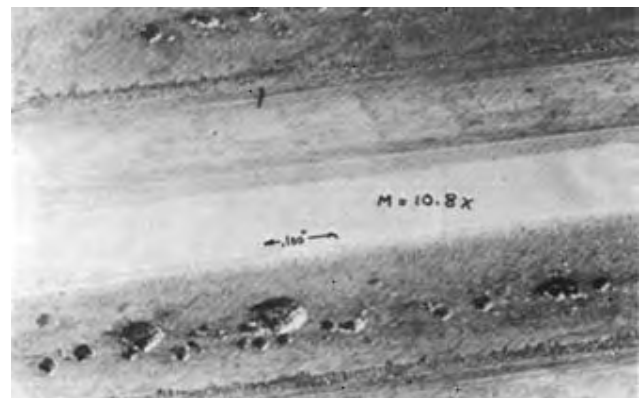
FIG. 2.4 (683-9) INITIAL (CORRECTIVE) PITTING ENLARGED PHOTO
