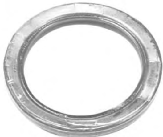
FIG. 5.3 (2342-38C) DAMAGED SEAL CASE
