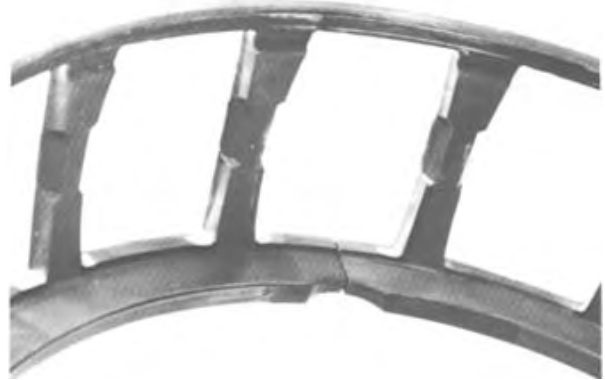
FIG. 4.6 (2342-33C) CAGE BREAKAGE AT NOTCH AND REDUCED SECTION
