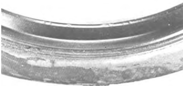
FIG. 5.6 (2342-41C) BLISTERS ON SEAL LIP
