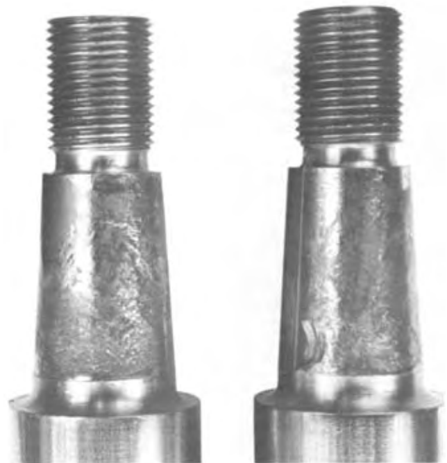
FIG. 3.7 (2342-27C) FRETTING CORROSION
