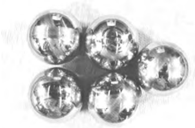
FIG. 4.4 (2342-31 C) BALL BANDING
