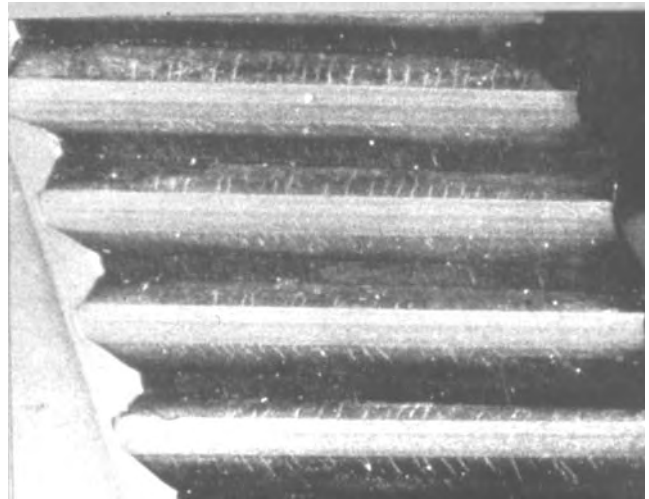
FIG. 2.48 (2342-23C) GRINDING CRACKS (ENLARGED)
