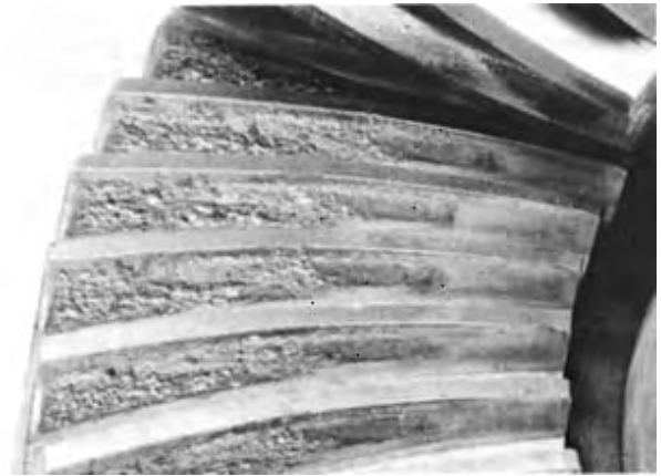
FIG. 2.8 (2342-2C) DESTRUCTIVE (PROGRESSIVE) PITTING
