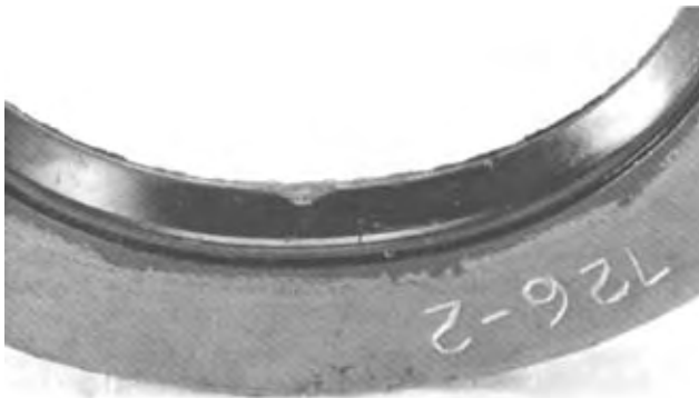
FIG. 5.5 (2342-40C) CHIPPING OF SEAL LIP
